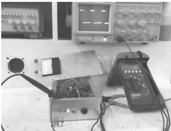
Figure 4. The oscilloscope showing 10% duty cycle with the green LED lit up indicating it is charging.
